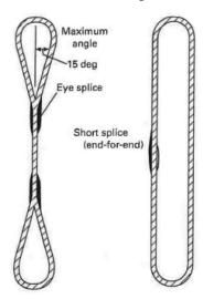
Figure 23 Synthetic Fiber Rope Slings
